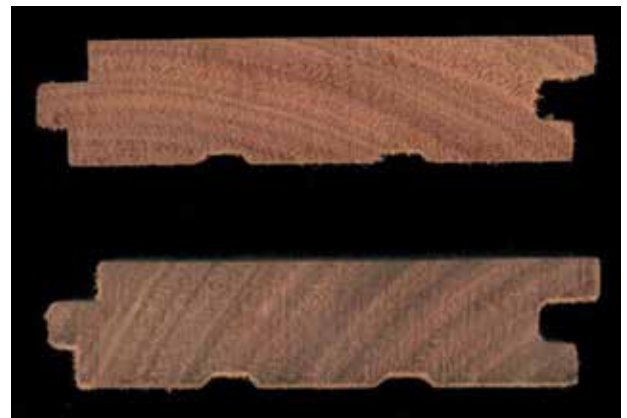
Backsawn and quartersawn floorboards.
