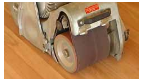
Third pass of sanding in the board direction.
