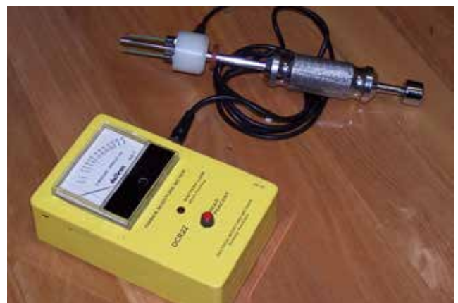
Resistance moisture meter - Measures moisture between the pins – Need to correct reading for temperature and species.
