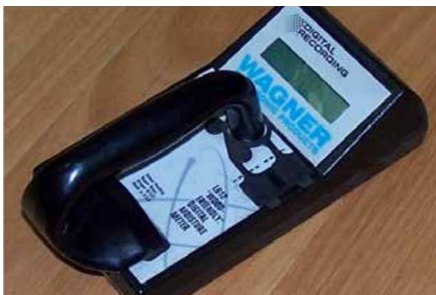
Capacitance moisture meter - Measures average moisture – Need to set species density.
