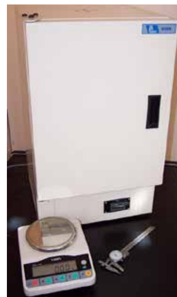
Oven dry testing – Provides the most accurate moisture content test.
